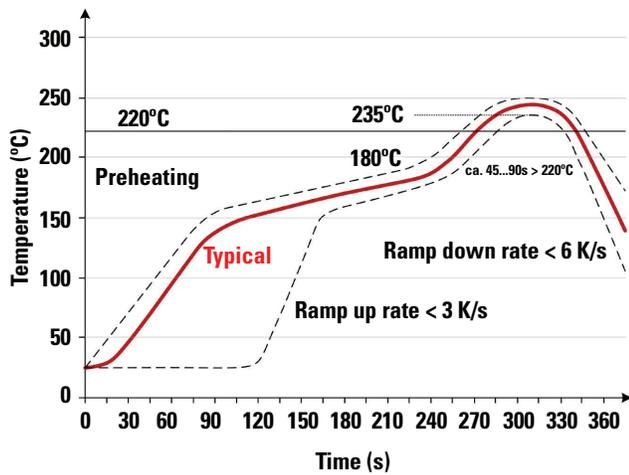
Soldering process: Depending on the application, this component is suited to the following methods:
